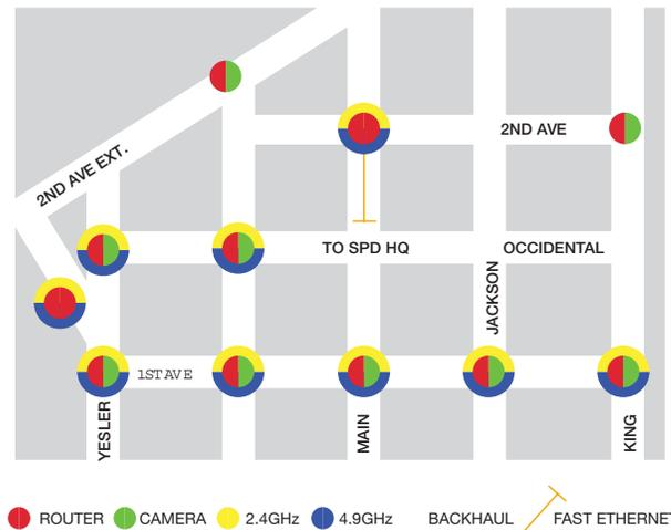
*A quad-radio MSR4000 tri-band wireless mesh router receives video signals from nine cameras deployed over a five-block area and centralizes them in the Seattle Police Department video surveillance center. The video is then sent to a mobile command center and can be viewed on handheld devices carried by patrolling officers.*
