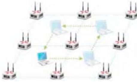
Figure 6: With MobileMatrix, users are free to move about the entire wireless mesh without reinitiating active sessions because the seamless transition from one AP to another is completed in less than 50 milliseconds.
