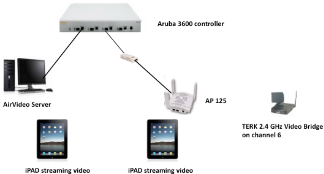
Figure 3a – The configuration for Test 3, which evaluated Aruba’s remediation capabilities when faced with interference from the Terk transmitter. Source: Aruba Networks/Farpoint Group.
