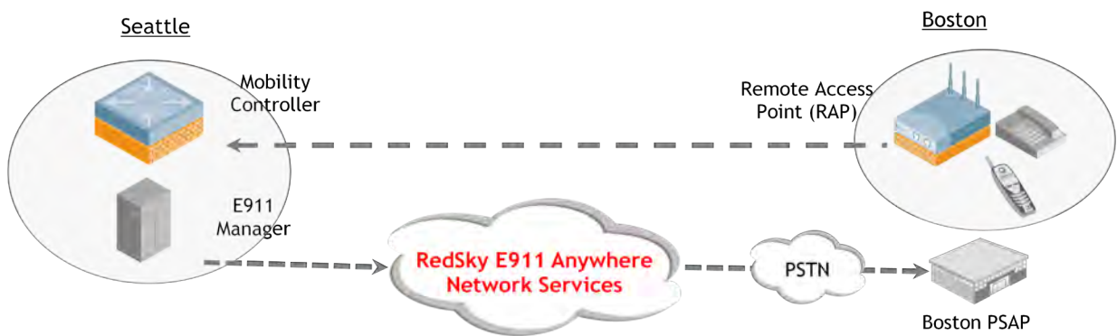
An emergency call on a RAP is re-directed to the correct PSAP via RedSky E911 Anywhere Network Services
