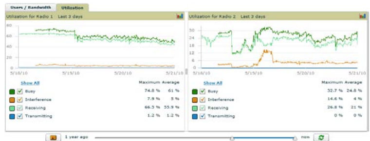
Figure 4. Channel utilization metrics in AirWave 7.
