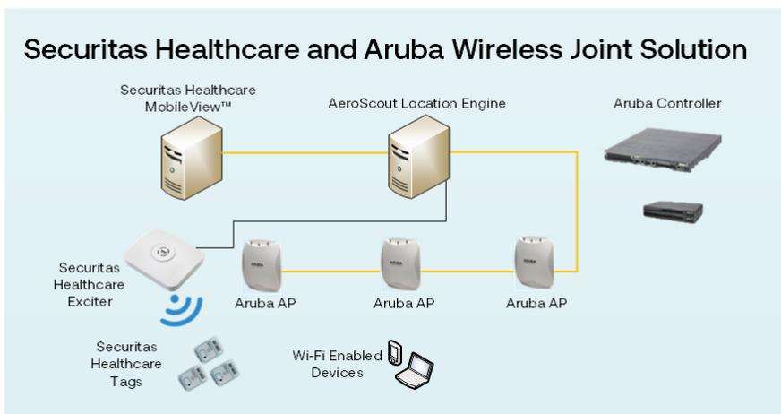
The AeroScout-Aruba joint solution can work with **IBSS** and **WDS**.
