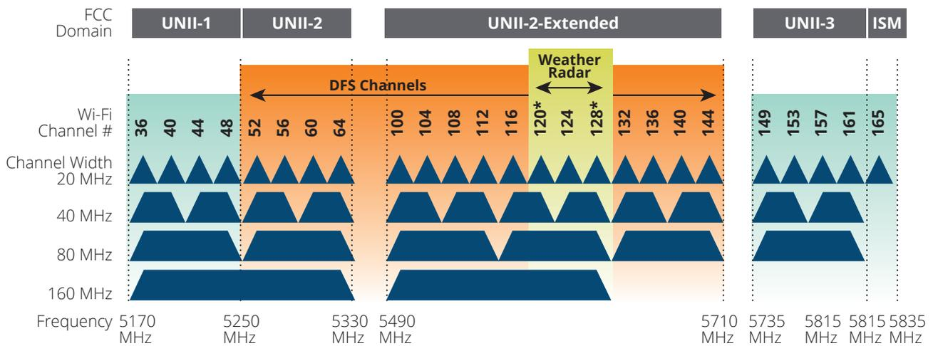
Figure 3: 5GHz channel allocation in North America
