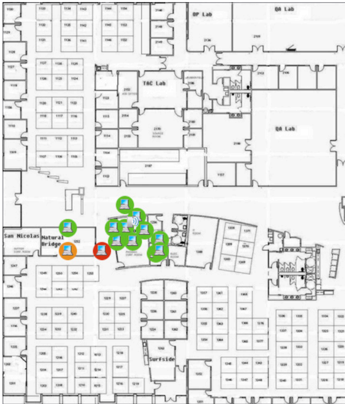
Figure 2: This floor plan shows an unhealthy client (red), which ClientMatch will automatically steer to a better AP and radio to optimize overall performance.
