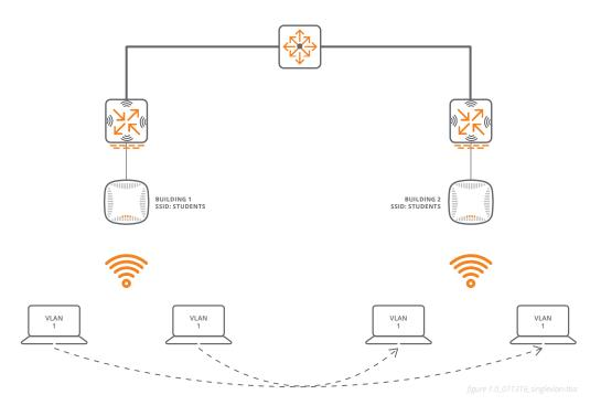
Figure 1: Single VLAN Design
