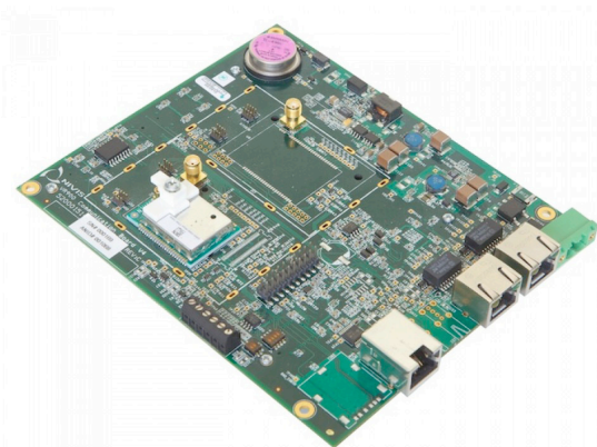
Figure 5: Control Data Systems VR800 WirelessHART/ISA100a VersaRouter Gateway Card
