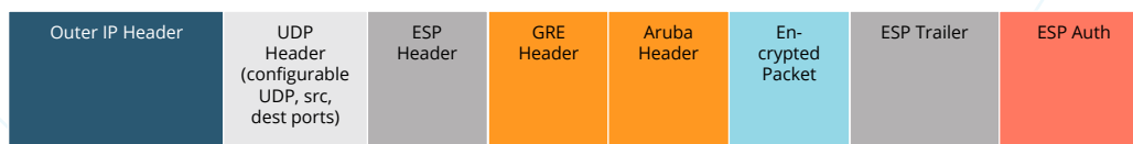
Figure 10. IPsec UDP (ESP) packet with Aruba encapsulation
