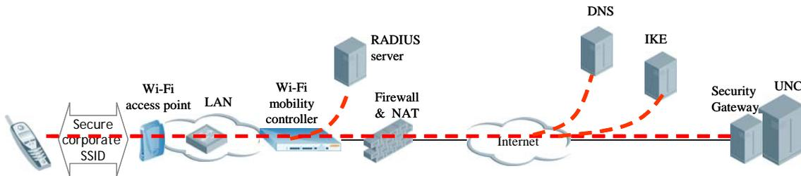
The diagram above shows the functional entities required for secure UMA service over a corporate WLAN.
