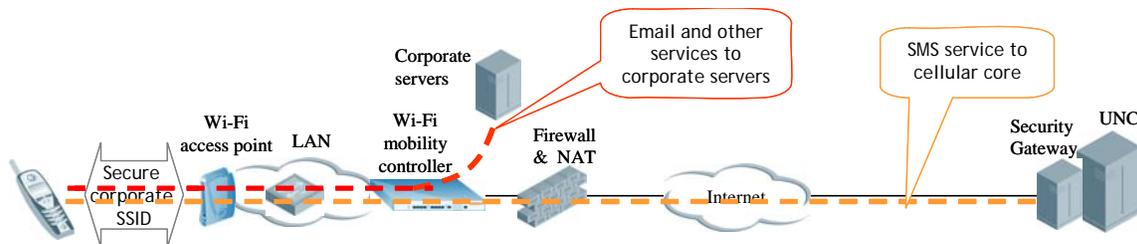
However, some UMA phones now allow for non-operator mobile data services, such as email or Web browsing, to be directed outside the UMA service tunnel and directly to servers on the corporate network or the Internet. The diagram above shows how this works. Note that the phone has one Wi-Fi association on a single SSID, but maintains two or more traffic streams.
